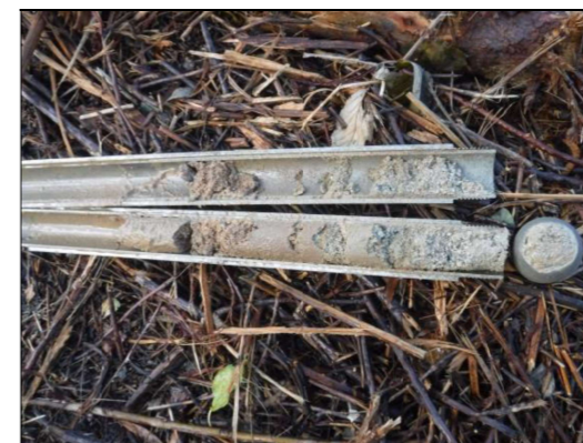
Foto 3: Sondeig S-2, SPT a 1,0 metre.
